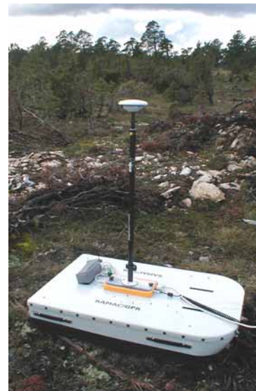
Typical field setup. On the MALÅ shielded antenna the GPS equipment is mounted, elevated above the radar antenna.
