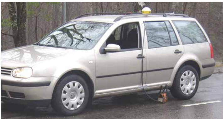
The GPR system mounted in a car, with the GPR antenna underneath the rear door and the GPS antenna on the roof.
