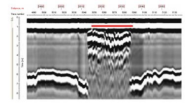
The next example clearly shows the radar ability to detect even small-scale changes in the ice. In this case a part of the ice, approximately 3 m along the measured profile (marked red), indicates an area with thinner ice.
