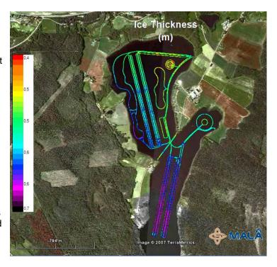
During the test season the lake ice tracks is scanned regularly with GPR. In this example the total measuring length was 25 km and takes around 2 hours from start of the measurements until the final map is produced and distributed. This is very cost- and time-saving compared with conventional drilling and measuring. The measurements and production of ice thickness maps is performed by one person only and no special expertise is needed.
